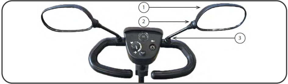
Figure 3. Delta steering column and rear-view mirrors
